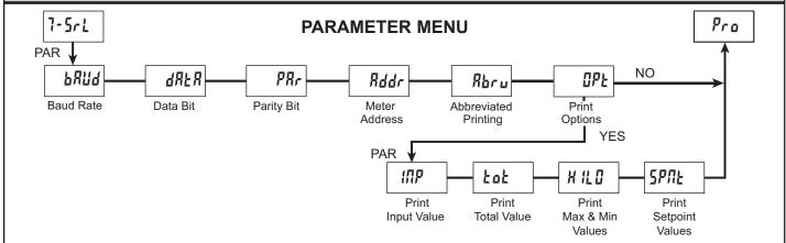
It is necessary to match the PAX meter's serial communications parameters to the host's parameters before communications can be established. This is accomplished by using the PAX front panel keys to enter 7-5rt.
